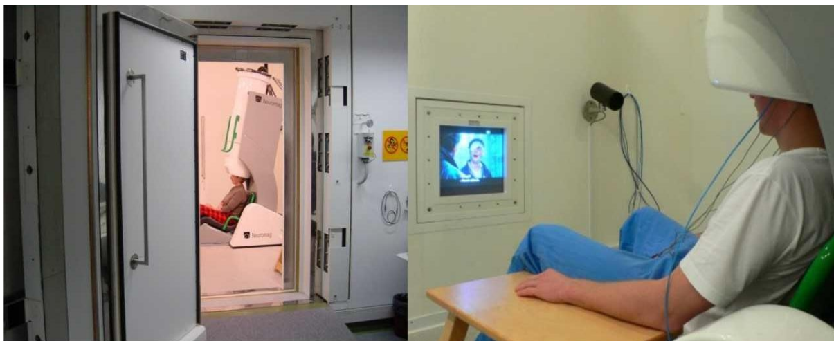
Fig. 10: MEG measurement: Shielded measurement cabin in the biomagnetism section of the Neurological Clinic in Heidelberg and test person during measurement (image source: Peter Schneider)
